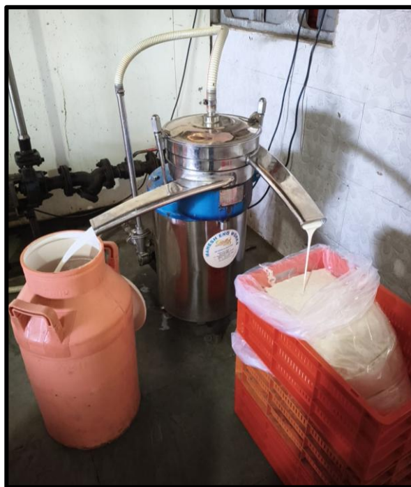
Fat Separator Unit
